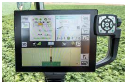
Tractor-mounted sensors can monitor crop nutrition requirements in real time and adjust dose rates to match their precise needs
